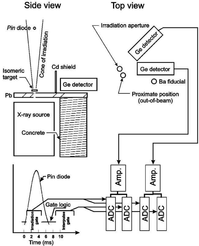
FIG. 1. Schematic drawing of the experimental arrangement showing the geometric placements and dimensions of the components, together with timing and arrangement of the electronics.
