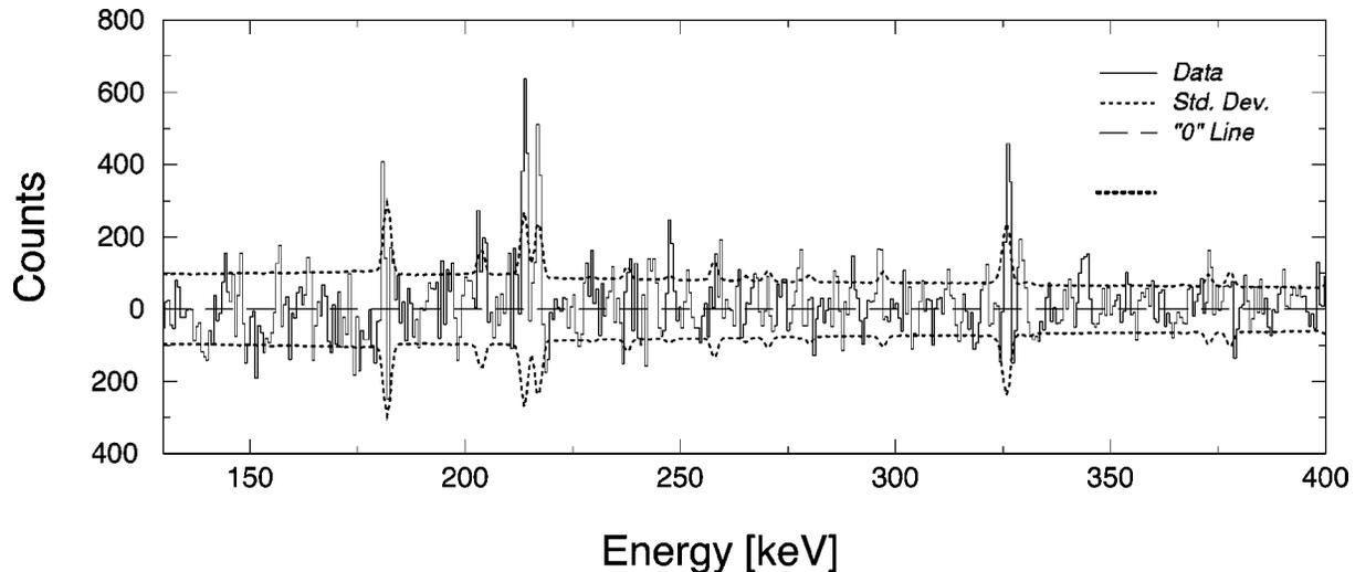
FIG. 4. Plot of the differences in counts obtained in the spectrum of the  $^{178}\text{Hf}$  from the isomeric target acquired with the detector connected to the 2K ADC's. Curves showing computed values for  $1\sigma$  for the differences are shown by the dotted lines.
