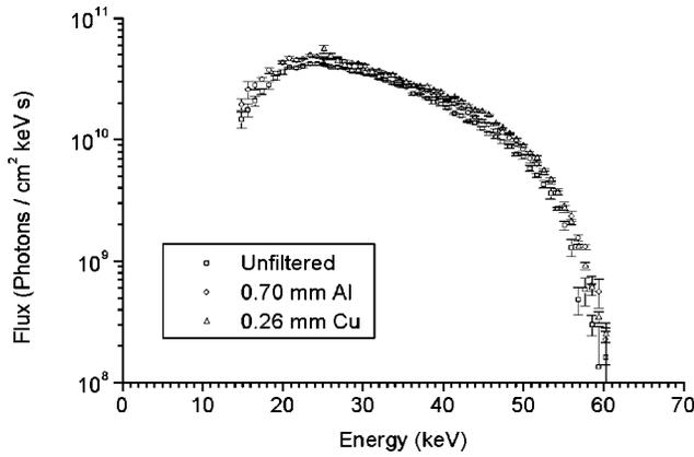
FIG. 2. Graph of the x-ray spectral flux expected at the inbeam position of the isomeric target. These experimental data for a 63 keV endpoint were measured with a Ge detector from input attenuated with a pin hole and placed at 12 m distance from the x-ray tube.
